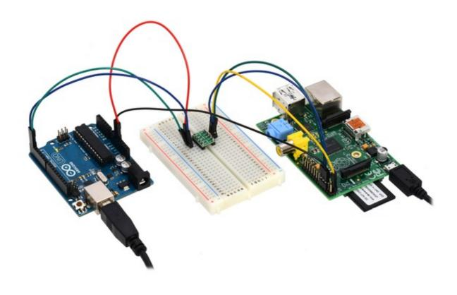
Using the 4-channel bidirectional logic level shifter to create a serial connection between a 5 V Arduino Uno and a 3.3 V Raspberry Pi.
