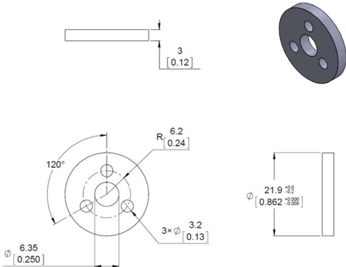
Mechanical drawing of the Pololu aluminum scooter wheel adapter flat washer. Units are mm over [inches].
