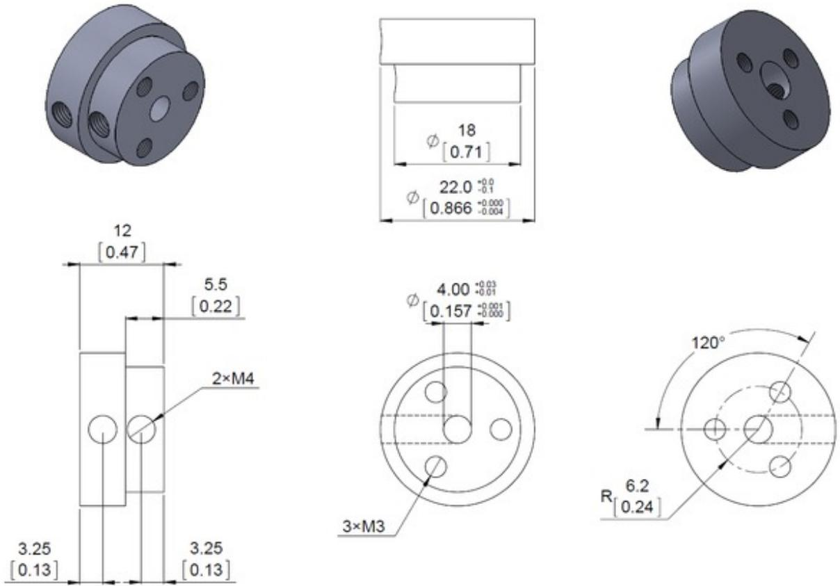
Mechanical drawing of the Pololu aluminum scooter wheel adapter threaded mount for 4 mm shafts. Units are mm over [inches].
