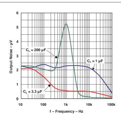
Figure 26. LP2951 Output Noise vs Frequency
