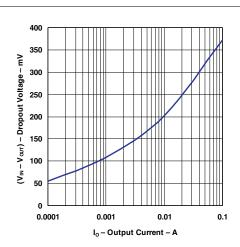
Figure 13. Dropout Voltage vs Dropout Current
