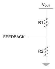
Figure 32. Adjusting the Feedback on the LP2951
