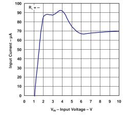
Figure 2. Input Current vs Input Voltage ( $R_L = OPEN$ )
