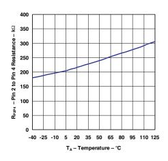
Figure 27. LP2951 Divider Resistance vs Temperature
