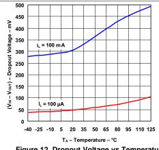
Figure 12. Dropout Voltage vs Temperature
