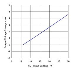
Figure 30. Line Regulation vs Input Voltage
