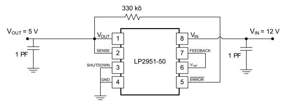
Figure 33. 12-V to 5-V Converter
