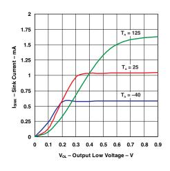
Figure 17. LP2951 ERROR Comparator Sink Current vs Output Low Voltage
