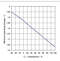
Figure 14. LP2951 Minimum Operating Voltage vs Temperature
