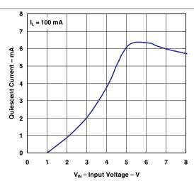
Figure 8. Quiescent Current vs Input Voltage (I<sub>L</sub> = 100 mA)
