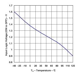
Figure 29. Shutdown Threshold Voltage (On to Off) vs
