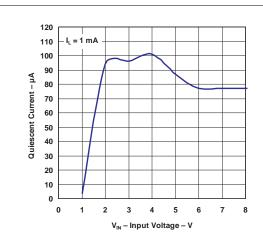
Figure 7. Quiescent Current vs Input Voltage (I<sub>L</sub> = 1 mA)
