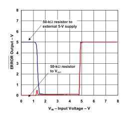
Figure 16. LP2951 ERROR Comparator Output vs Input Voltage
