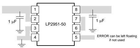
Figure 35. LP2951 Layout Example (D or P Package)
