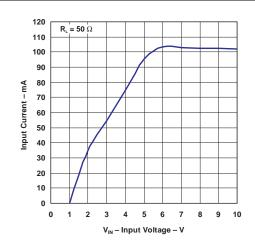
Figure 4. Input Current vs Input Voltage ( $R_L = 50 \Omega$ )
