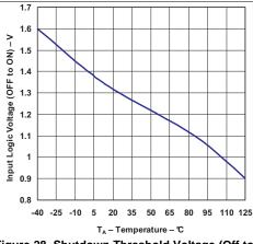
Figure 28. Shutdown Threshold Voltage (Off to On) vs
