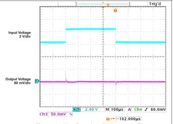
Figure 18. Line Transient Response vs Time
