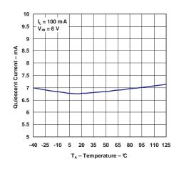
Figure 9. Quiescent Current vs Temperature (I<sub>L</sub> = 100 mA)
