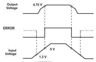
Figure 31. ERROR Output Timing
