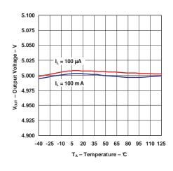
Figure 5. Output Voltage vs Temperature
