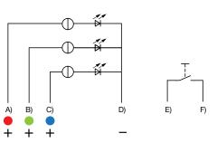
A) Cable (color of the LED), Supply voltage B) Cable (color of the LED), Supply voltage
