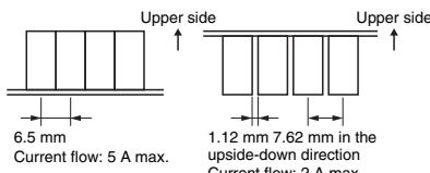
Note. The space between each relay required for heat radiation may vary with operating conditions. Contact your OMRON representative for details.
