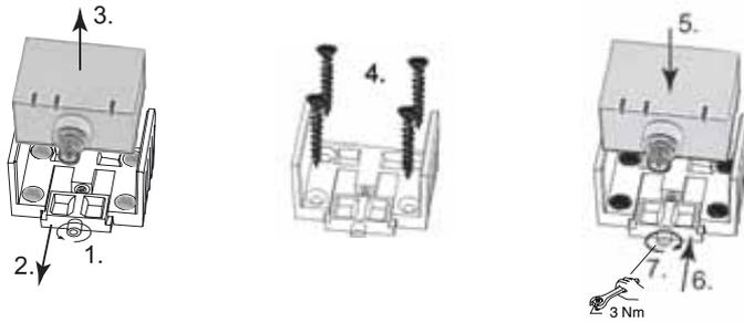
1. Loosen the central screw under the sensor connection.
