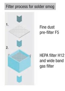
Filter process for solder smog and wide band gas
