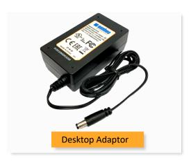
The AMA24D-Y is a small industrial grade desktop adapter. Offering a commercial input voltage range of 90-264VAC and with maximum output power of 24W. This adapter will offer many benefits to powering your system such as low power consumption, high efficiency (meets Erp Tier 2/DOE VI), meeting IEC62368-1, FCC, Class B, CISPR32, Class B.
