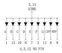
Internal Circuit Diagram (Common Cathode)
