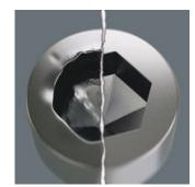
Hexagon screws can endure a problem because the contact surfaces delivering the power from the conventional tool, is transferred to the screw via very small surface areas. The consequence: the screw become damaged (rounding out). Hex-Plus tools have a greater contact surface that prevents this from happening! At the same time, as much as 20 % more torque can be applied. Good to know: Hex-Plus tools fit into every standard hexagon socket screw!
