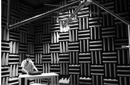
Acoustic radio wave anechoic chamber
