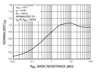
Figure 9. Normalized tooff vs. RBE
