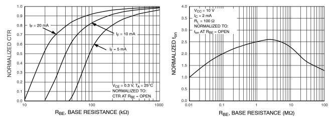
Figure 7. CTR vs. R<sub>BE</sub> (Saturated)
