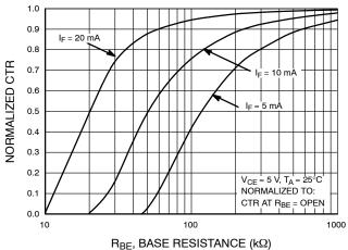
Figure 6. CTR vs. RBE (Unsaturated)
