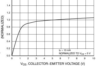
Figure 4. Output Current vs. Collector-Emitter Voltage
