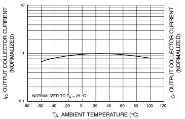
Figure 3. Output Current vs. Ambient Temperature
