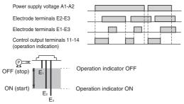
• When the liquid level falls to E2 (indicator turns ON), the pump starts. When the liquid level rises above E1 (indicator turns OFF), the pump stops.
