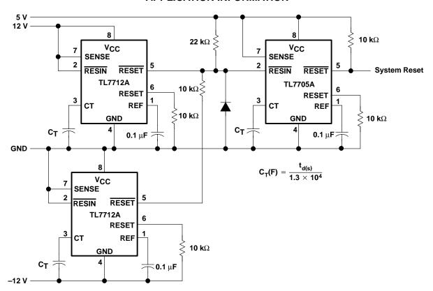
Figure 6. Multiple Power-Supply System Reset Generation
