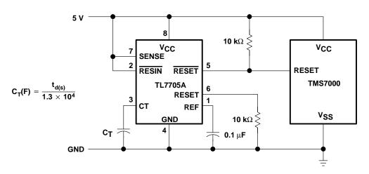
Figure 7. Reset Controller for TMS7000 System
