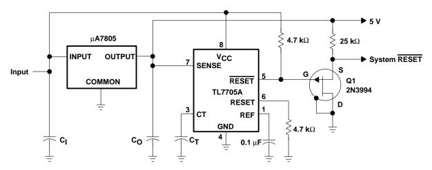
Figure 8. Eliminating Undefined States Using a P-Channel JFET
