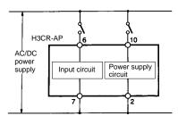
Since the input circuit and the power supply circuit are configured independently, the input circuit can be turned ON or OFF irrespective of the ON/OFF state of the power supply.
