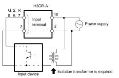
The H3CR-A $\square$ /-A $\square$ S/AP's power supply terminal 2 is a common terminal for input signals to the Timer. Do not disconnect the wires on terminal 2, otherwise the internal circuitry of the Timer will be damaged.
