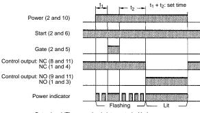
Gate signal (The operation is interrupted with the gate signal if the Timer detects an abnormal signal.)
