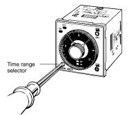
For ON-time, the desired time unit (sec, 10 s, min, and hrs, or 10 s, 10 min, hrs, and 10 h) is indicated in the ON-time unit display window at the lower right corner of the front panel and can be changed by turning the ON-time unit selector located below the ON-time unit display window.
