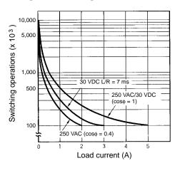
Reference: A maximum current of 0.15 A can be switched at 125 VDC  $(\cos\phi = 1)$ and a maximum current of 0.1 A can be switched if L/R is 7 ms. In both cases, a life of 100,000 operations can be expected. The minimum applicable load is 10 mA (100 mA for H3CR-A8E) at 5 VDC (failure level: P).
