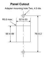
The mounting panel thickness Note: should be 1 to 3.2 mm.
