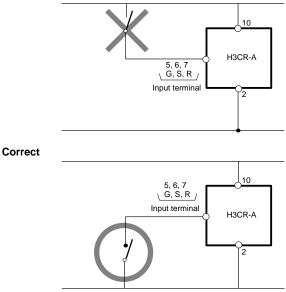
Do not connect a relay or any other load between input terminals, otherwise the internal circuit of the Timer will be damaged due to the high-tension voltage applied to the input terminals.
