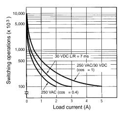
Reference: A maximum current of 0.15 A can be switched at 125 VDC (cos = 1) and a maximum current of 0.1 A can be switched if L/R is 7 ms. In both cases, a life of 100,000 operations can be expected. The minimum applicable load is 10 mA at 5 VDC (failure level: P).
