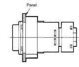
Note: The adapters for two or more timers mounted in a vertical line are different in orientation from those mounted in a horizontal line.
