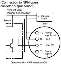
**Note:** The input circuit is isolated from the power supply circuit. Thus, an NPN transistor can be connected.
