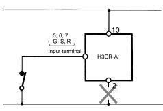
Make sure that the voltage is applied within the specified range, otherwise the internal elements of the Timer may be damaged.
