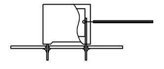
Temperature monitored inside the capacitor.
