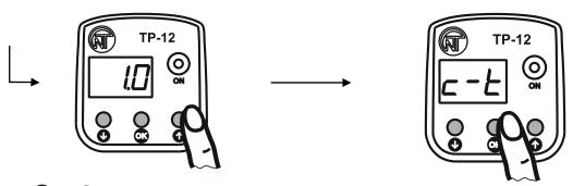
Via or pushbutton change parameter value within -5.0 to +5.0 °C with increment size of 0.1 °C
