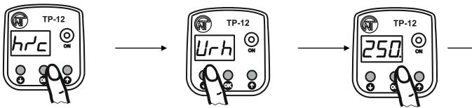
Hold **OK** pushbutton pressed for 3 seconds until the display shows «hr'c» menu parameter
