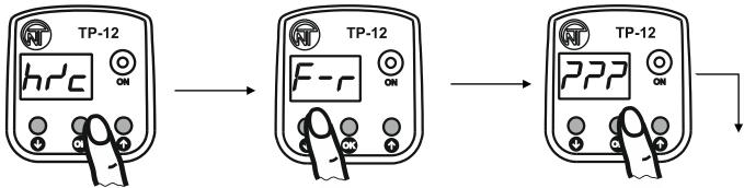
Hold **OK** pushbutton pressed for 3 seconds until the display shows «hrc» menu parameter
