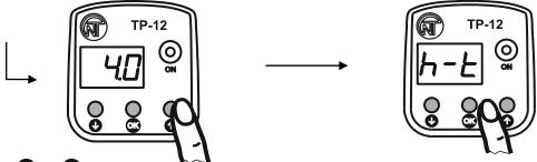
Via or pushbutton change parameter value within 0.1 to 30 °C with increment size of 0.1 °C
