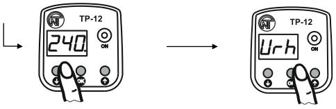
Via or pushbutton change parameter value within 230 to 290 V with increment size of 5 V
