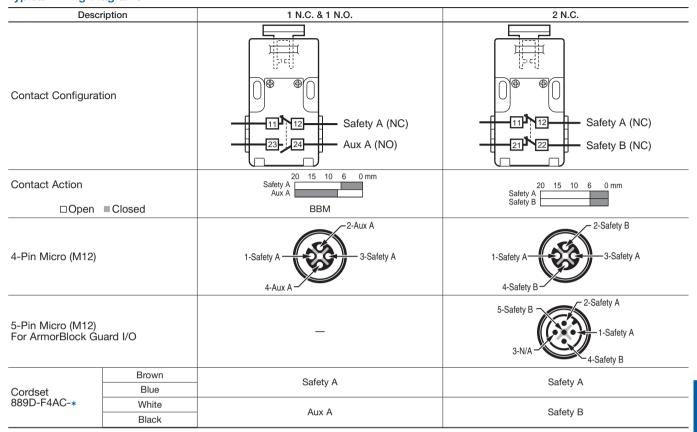
$<sup>\</sup>boldsymbol{*}$  Replace symbol with 2 (2 m), 5 (5 m) or 10 (10 m) for standard cable lengths.
