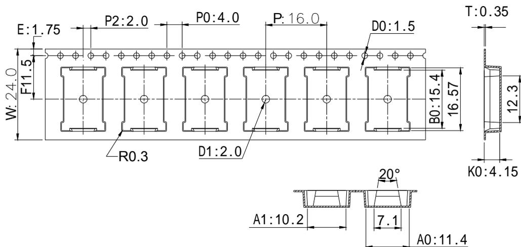
Note: Tolerances unless mentioned  $\pm 0.25$ mm. Unit = mm
