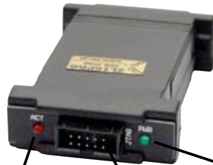
PWR LED – signalling the proper value of power supply voltage
