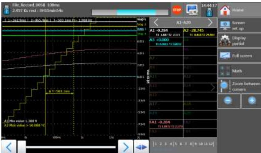
When waiting for the trigger, the screen makes it possible to display the channels in real time (scrolling mode); you can select the scrolling rate.
