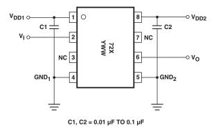
Figure 10. Recommended printed circuit board layout.
