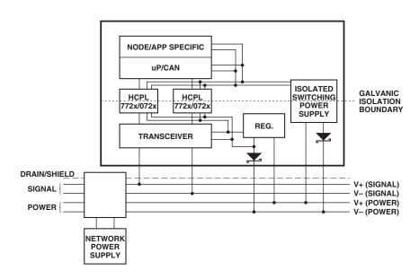
Figure 18. Isolated node powered by the network.
