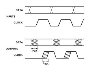
Figure 14. Parallel data transmission example.
