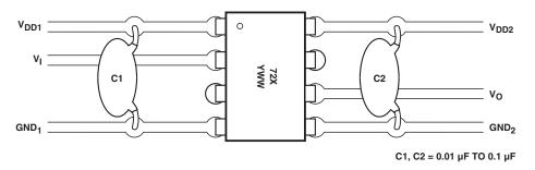
Figure 11. Recommended printed circuit board layout.
