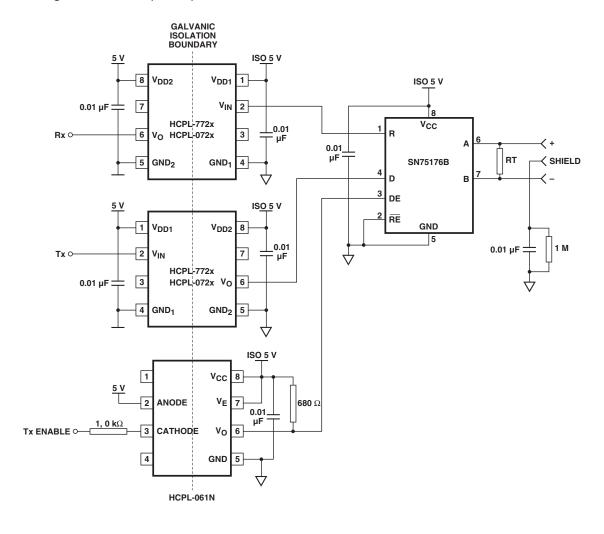
Figure 23. Recommended PROFIBUS application circuit.
