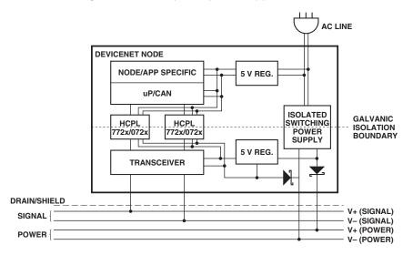
$\label{eq:Figure 20.} \textbf{Isolated node providing power to the network.}$
