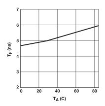
Figure 6. Typical fall time vs. temperature.
