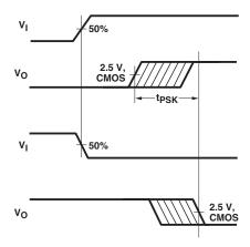
Figure 13. Propagation delay skew waveform.
