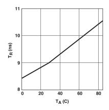
Figure 5. Typical rise time vs. temperature.
