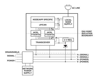
Figure 16. Typical DeviceNet Node.
