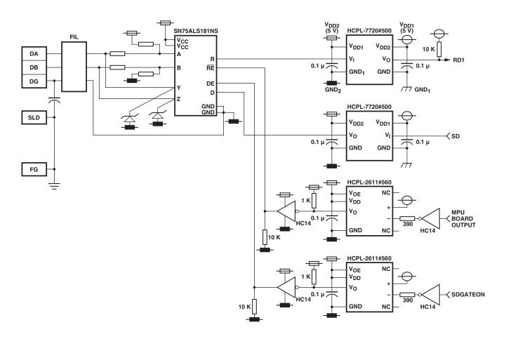
Figure 17. Recommended CC-Link application circuit.
