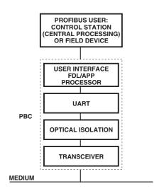
Figure 22. PROFIBUS Controller (PBC).
