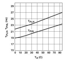
Figure 3. Typical propagation delays vs. temperature.
