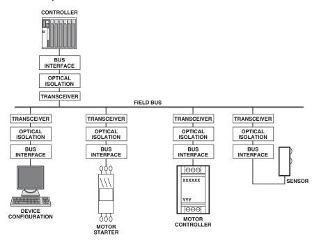
Figure 15. Typical field bus communication physical model.
