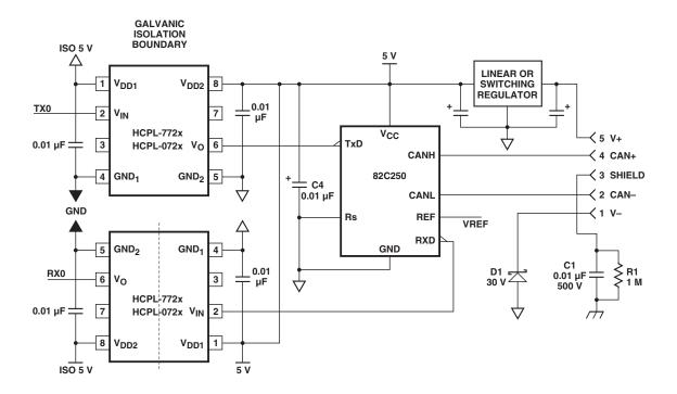
Figure 21. Recommended DeviceNet application circuit.
