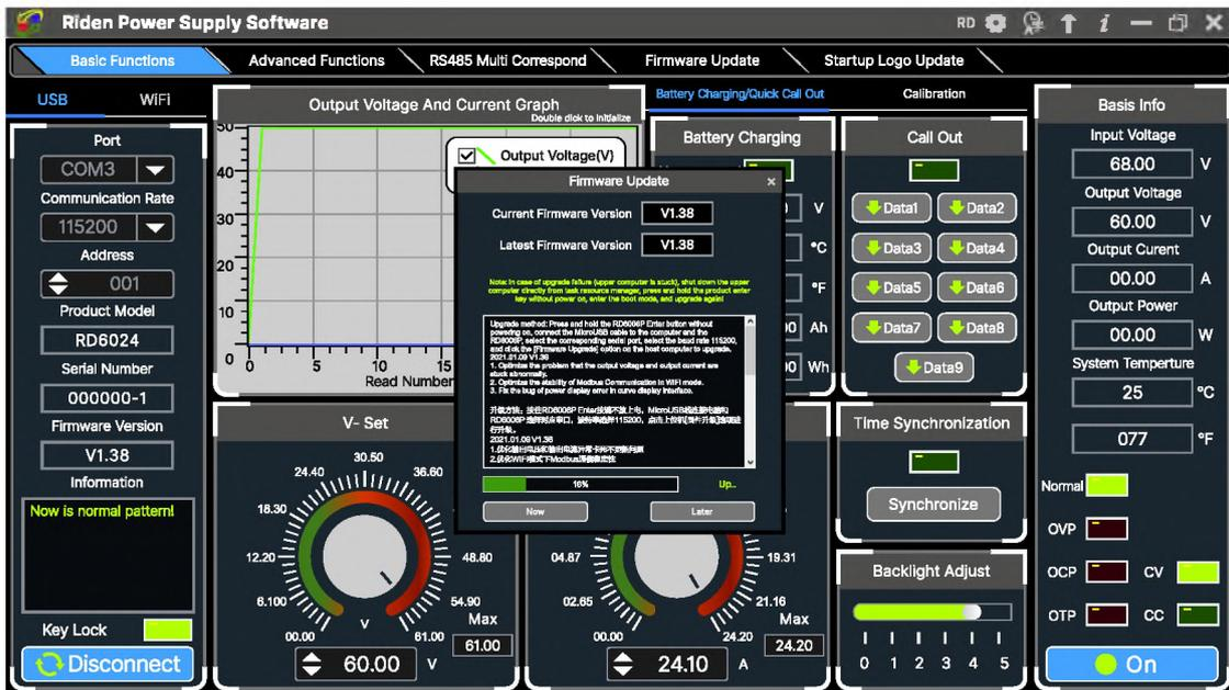
During the firmware upgrade process, the interface is displayed as follows:
