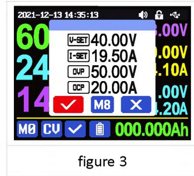
potentiometer to change the setting and press encoder potentiometer to return, it will be stored into **M0** automatically, or you go to the data group setting menu, change the setting and press encoder potentiometer to return, it will save too, and it will not save by other settings.
