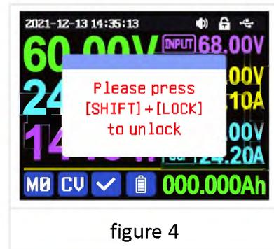
communication starts, there will be AO: Button lock status **🔒** displayed on the top (cannot unlock manually), at this time, the A: power button can be used, pressing other buttons will show(as shown in figure 4), the keypad will be automatically unlocked after 3 seconds when the communication disconnected, there will be AO: Button lock status **🔓** displayed.
