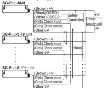
Note: For connecting multiple units, connect the check output line (gray) with the check input line (pink) of the **SG-P□□-S** sub unit connected next. Connect the check output line (gray) of the **SG-P□□-S** sub unit connected at the end with the check input line (pink) of the **SG-P□□-M** standard unit placed at the beginning.
