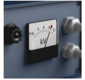
Each Kraftform Kompakt VDE set has been tested individually at 10,000 volts, in accordance with IEC 60900.This ten-times-higher testing load guarantees safe working at their maximum permitted load of 1,000 volts. Kraftform Kompakt VDE
