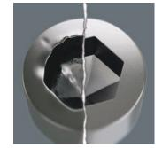
Hexagon socket screws are a problem, because the contact surfaces that transfer the force of the tool to the screw are very narrow. The consequence: the head of the screw can be damaged, usually rounding out the recess. Hex-Plus tools have larger contact surfaces to prevent this, driving from the flats of the recess, rather than the corners. Good to know: Hex-Plus tools fit into every standard hexagon socket screw!
