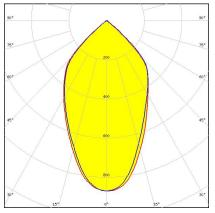
Dimensions: 82.0 mm x 82.0 mm Height: 31.00 mm ~50° wide beam compatible with BJB connectors
