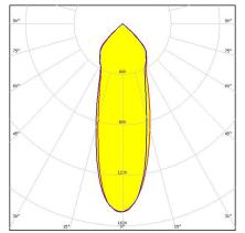
Dimensions: 82.0 mm x 82.0 mm Height: 31.00 mm ~30° medium beam
