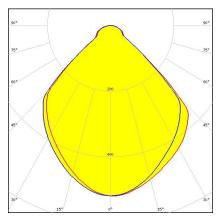
Dimensions: 82.0 mm x 82.0 mm Height: 31.00 mm White version with ~91° wide beam
