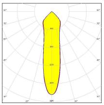
Dimensions: 82.0 mm x 82.0 mm Height: 31.00 mm ~20° spot beam compatible with BJB connectors
