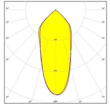
Dimensions: 82.0 mm x 82.0 mm Height: 31.00 mm ~30° medium beam compatible with BJB connectors
