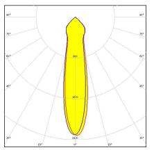
Dimensions: 82.0 mm x 82.0 mm Height: 31.00 mm ~20° spot beam
