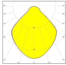
Dimensions: 82.0 mm x 82.0 mm Height: 31.00 mm White version with ~91° wide beam compatible with BJB connectors
