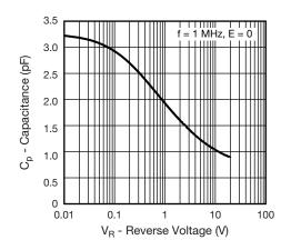
Fig. 4 - Diode Capacitance vs. Reverse Voltage
