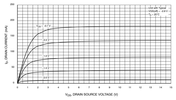
Figure 3. Common Drain–Source, J109
