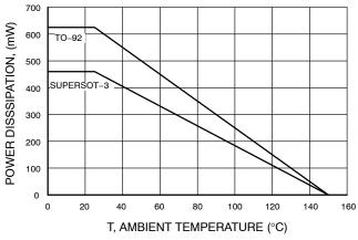
Figure 12. Power Dissipation vs. Ambient Temperature
