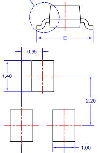
LAND PATTERN RECOMMENDATION\* \*FOR ADDITIONAL INFORMATION ON OUR Pb-FREE STRATEGY AND SOLDERING DETAILS, PLEASE DOWNLOAD THE ON SEMICONDUCTOR SOLDERING AND MOUNTING TECHNIQUES REFERENCE MANUAL, SOLDERRM/D.
