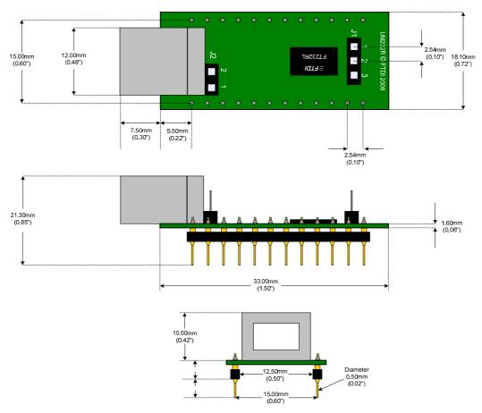
Figure 4.1 UM232R Module Dimensions
