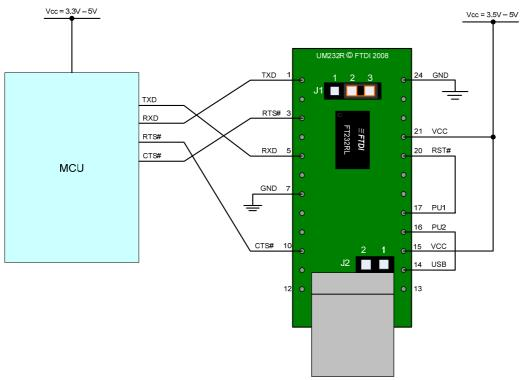
Figure 6.2 Self-Powered Configuration
