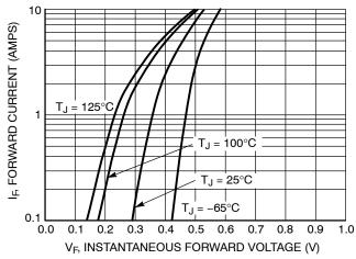
Figure 1. Typical Forward Voltage
