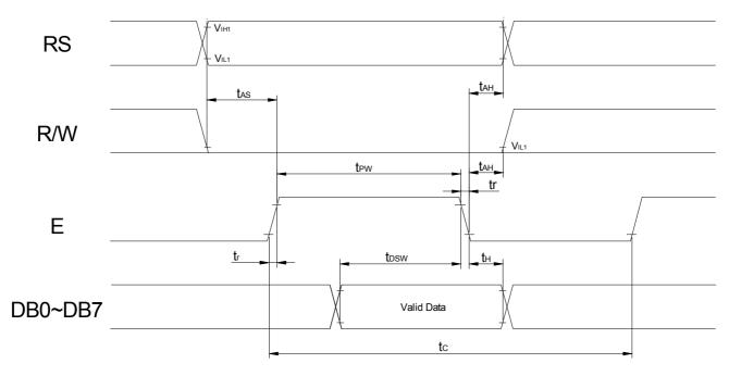
10-2-2 Read Mode (Reading Data from ST7066 to MPU)
