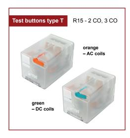
**Test buttons (no latching)** are recommended for R2N...WT, R3N...WT, R4N...WT, R15...WT 2 CO, R15...WT 3 CO relays - **for applications that do not allow permanent contact latching**. By manual operation (pressing the button) relay contacts can get switched for as long time as long the button is pressed. Contacts return to initial position as soon as pressure is released from the button. Those operations can be done while the coil is deenergized.
