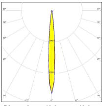
Dimensions: 49.9 mm x 49.9 mm Height: 23.90 mm ~15° spot beam
