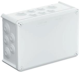
All the T series junction boxes are UV-resistant. They are made of a thermoplastic polypropylene plastic with plug-in seals made of ethylene vinyl acetate (EVA). This plastic is soft, which means that it is malleable. This allows installation of cables through the 16 x M32
