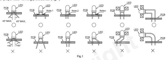
Correct mounting method "X" Incorrect mounting method
