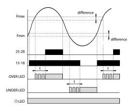
After the supply (monitored) voltage is connected, the green LED is on.
