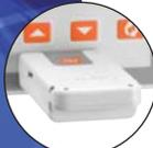
Through the optical port, direct connection to a PC USB port (using CX 01) or via WiFi (using CX 02) is allowed. CX 02 dongle (WiFi) can furthermore make:
