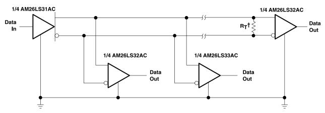
$<sup>^{\</sup>dagger}$  RT equals the characteristic impedance of the line.
