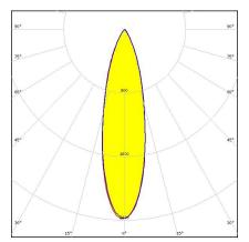
Dimensions: 9.9 mm x 9.9 mm Height: 6.60 mm ~20° medium beam optimized for LUXEON Rebel. 6.6 mm high variant with clip installation.
