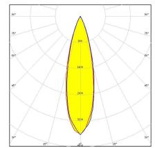
Dimensions: 9.9 mm x 9.9 mm Height: 6.60 mm ~20° medium beam optimized for Osram
