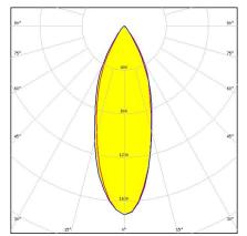
Dimensions: 9.9 mm x 9.9 mm Height: 6.60 mm ~35° wide beam optimized for Osram Oslon SSL 80. 6.6 mm high variant with location pin installation.
