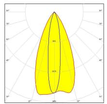
Dimensions: 9.9 mm x 9.9 mm Height: 6.60 mm ~45° x 20° oval beam optimized for LUXEON Rebel. 6.6 mm high variant with location pin installation.
