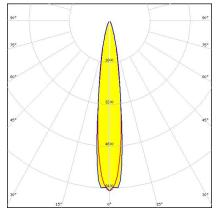
Dimensions: 9.9 mm x 9.9 mm Height: 6.80 mm ~19° spot beam. 6.8 mm high variant with location pin installation.
