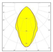
Dimensions: 9.9 mm x 9.9 mm Height: 6.60 mm ~80° wide beam optimized for Osram Oslon SSL 80. 6.6 mm high variant with clip installation.
