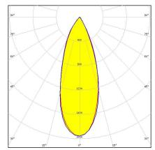
Dimensions: 9.9 mm x 9.9 mm Height: 6.80 mm ~35° wide beam. 6.8 mm high variant with location pin installation.
