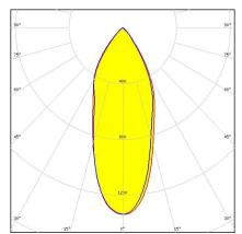
Dimensions: 9.9 mm x 9.9 mm Height: 6.81 mm ~45° wide beam optimized for Osram Oslon SSL 80. 6.8 mm high variant with location pin installation.
