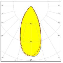
Dimensions: 9.9 mm x 9.9 mm Height: 6.80 mm ~45° wide beam optimized for CREE XP-E. 6.8 mm high variant with clip installation.
