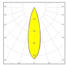
Dimensions: 9.9 mm x 9.9 mm Height: 6.80 mm ~20° medium beam. 6.8 mm high variant with location pin installation.
