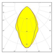
Dimensions: 9.9 mm x 9.9 mm Height: 6.65 mm ~80° wide beam optimized for Osram Oslon SSL 80. 6.6 mm high variant with location pin installation.
