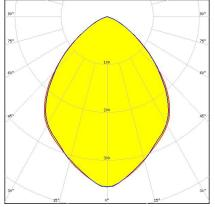
Dimensions: 9.9 mm x 9.9 mm Height: 7.00 mm ~80° wide beam optimized for CREE XP-E. 7.0 mm high variant with clip
