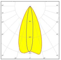
Dimensions: 9.9 mm x 9.9 mm Height: 6.80 mm ~45° x 20° oval beam. 6.8 mm high variant with location pin installation.
