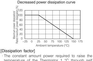
The constant amount power required to raise the temperature of the Thermistor 1 °C through self heat generation under stable temperatures.
