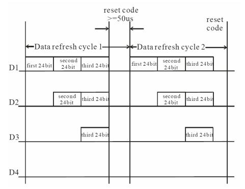
Note: The data of D1 is send by MCU, and D2, D3, D4 through pixel internal reshaping amplification to transmit.
