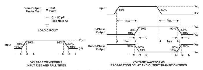
Figure 1. Load Circuit and Voltage Waveforms
