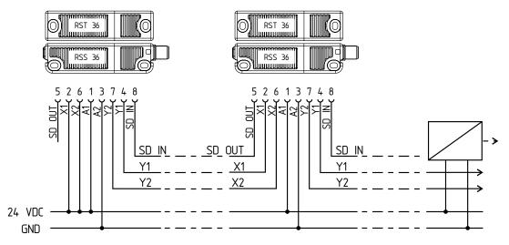
Y1 and Y2 = Safety outputs -> Safety-monitoring module SD-IN -> Gateway -> Field bus
