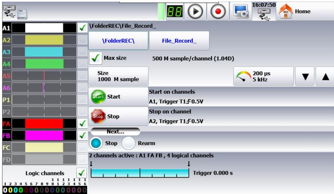
The program of triggers is different according to the pending mode (Direct, Memory, File or Template).
