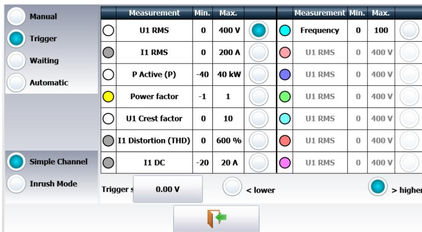
12.4.2.4. Trigger according to an inrush.
