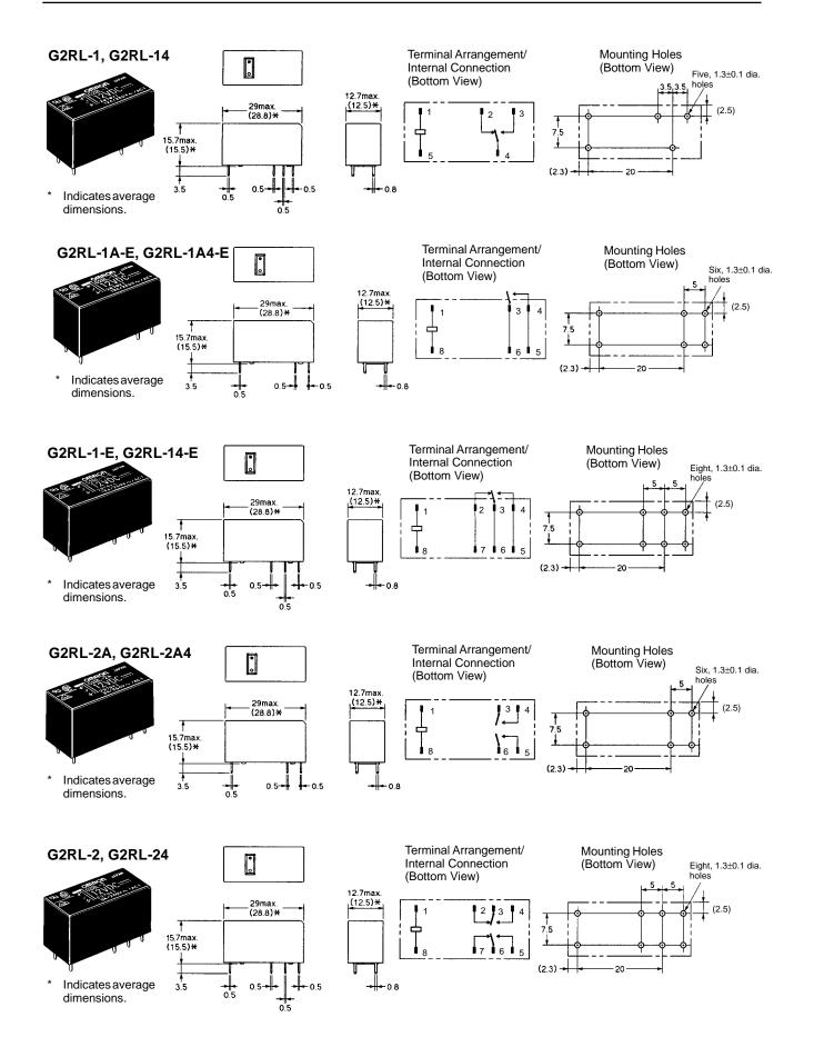
NOTE: DIMENSIONS SHOWN ARE IN MILLIMETERS. To convert millimeters to inches divide by 25.4.
