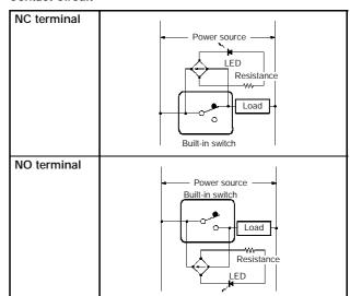
**Note:** If the wiring is as shown above, the operation of the respective parts will be as follows:
