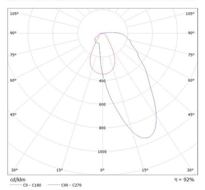
Luminaire: LEDiL Oy F15156\_RONDA-WAS\_(CXA1520) Lamps: 1 x Cree\_CXA1520\_(CXA1520-30F-N4-N0H-0001)\_982.885Im@250mA\_P=8.57638W\_I=0.250A
