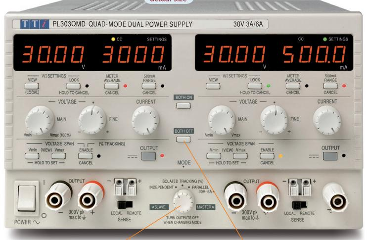
**Independent Mode:** The two outputs are completely independent and electrically isolated from each other.
