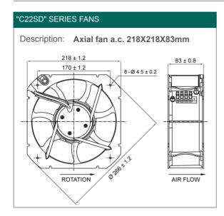
Fan material: casing of aluminium alloy die casting and fibre reinforced plastic (PA 6/6) impeller
